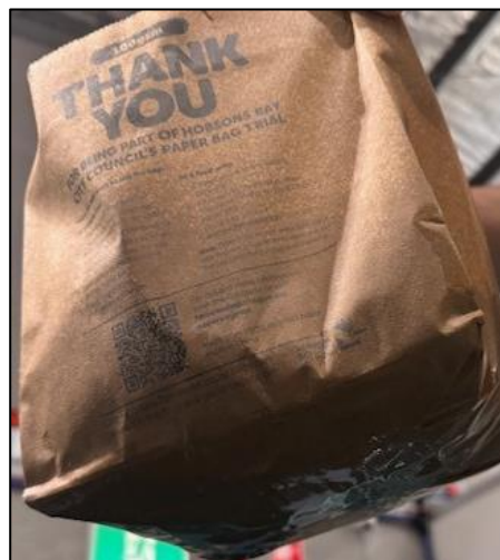
A 100GSM-weight paper caddy liner distributed by a Victorian council displayed degradation and significant leakage at Day 2 in lab tests.
